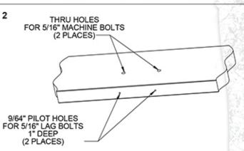
DRILL 5/16" THRU HOLES AND 9/64" X 1" DEEP PILOT HOLES
