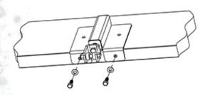
HOLD SPRING MOUNT IN PLACE AND INSTALL 5/16" LAG BOLTS AND WASHERS (2 PLACES)
